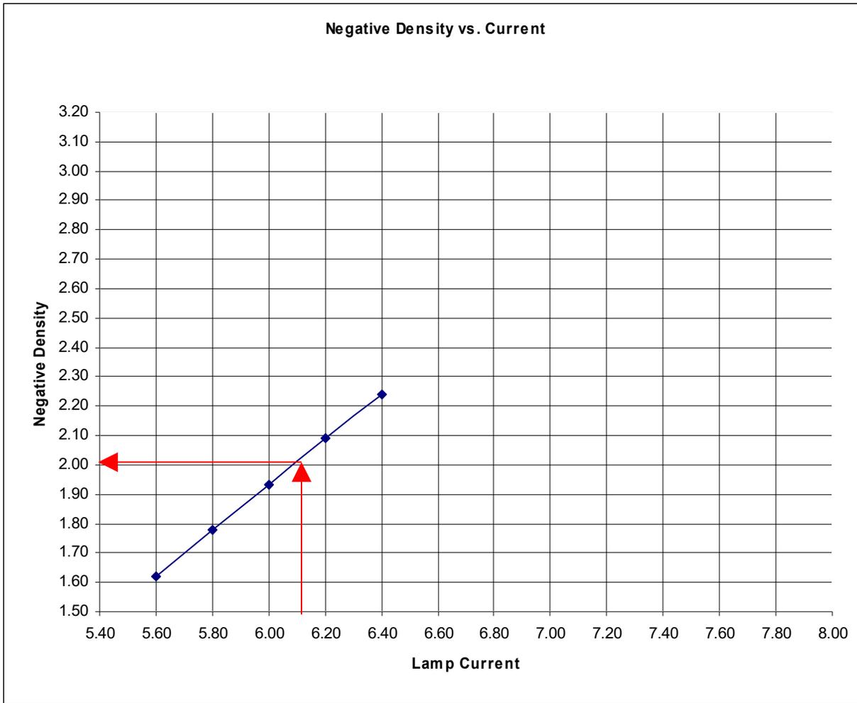
It should be noted that for high quality stereo optical recording, there should be a 0.05 ND or less difference in the negative film density between the left and right tracks (0.1 ND for dual bilateral mono tracks). The camera lamp balance should be checked regularly.
